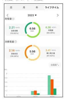
発電量=6.56Mwh=6,560kwh 自家消費量=2.21Mwh=2,210kwh 自家消費率=2,210÷6,560=33.7%
