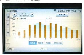
発電量=7,357.6kwh 売電量=3,979.3kwh 自家消費率= (7,357.6-3,979.3) ÷7,357.6 =45.9%
